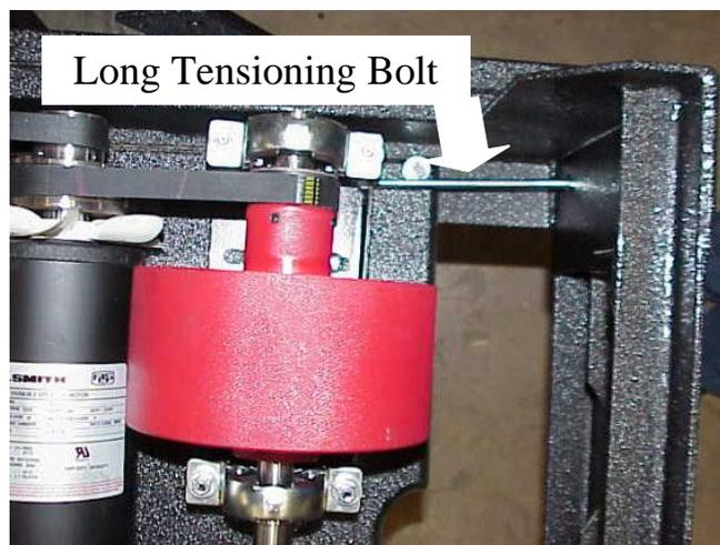
Use a ½” socket wrench to tighten the tensioning bolt just enough to remove the slipping. Check the tension on the belt that runs from the motor to the front roller by twisting or wiggling it.
